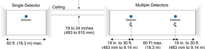
Detector positioning shown here is recommended for protected areas with flat ceilings. Spacing may vary for areas with high or sloped ceilings. In such cases, verify operation with smoke tests. In some cases potential smoke layering may be overcome by installing multiple beam detectors at different heights.
